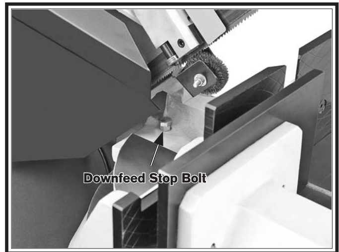
Figure 48. Adjusting downfeed stop bolt.
